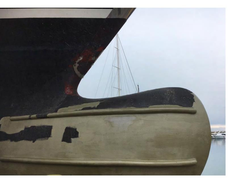
Fillers are usually applied by spatula or with a striker and may build-up high thicknesses. They are easy to sand and therefore suitable for restoring the original surface smoothness. Although they give a tough finish they are at the same time reasonably flexible to withstand cracking during the movement of the boat.
