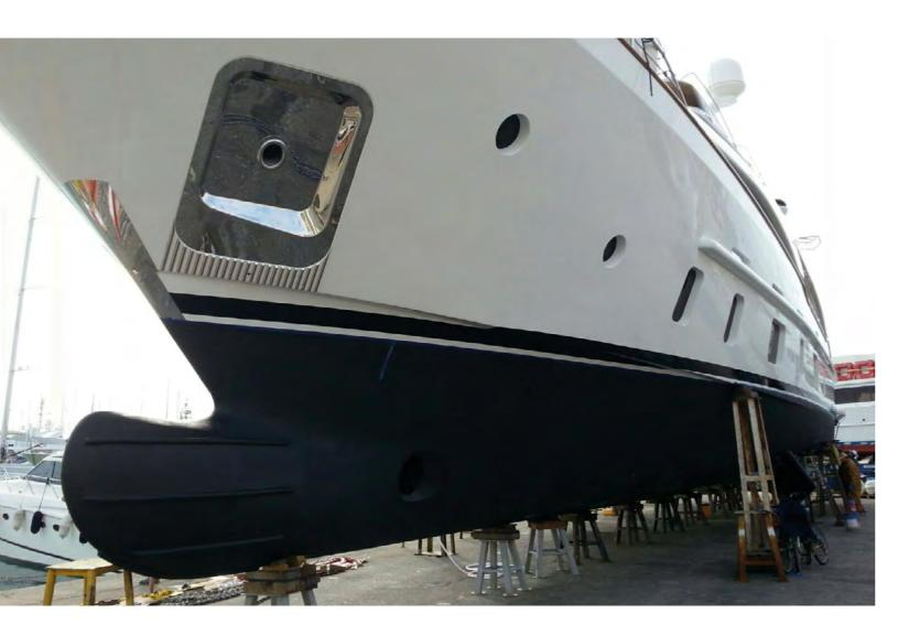
Without the protection of an effective antifouling paint the growth of vegetation and marine organisms can seriously impair the hull below the waterline, causing friction that decreases the speed of the boat and raising fuel consumption considerably. We must therefore remember the saying "those who spend more spend less" and avoid therefore to skimp and save on the cost and quality of the antifouling.
